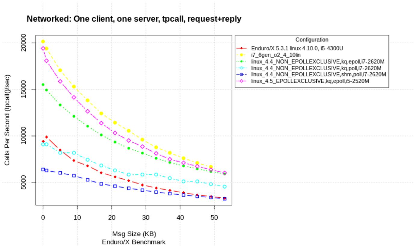
Here we see that network performance slightly fluctuate. That could be related with fact now bridge is involved to transfer the message over the network, and process count is bigger than CPU core count. Thus scheduler comes in work.
