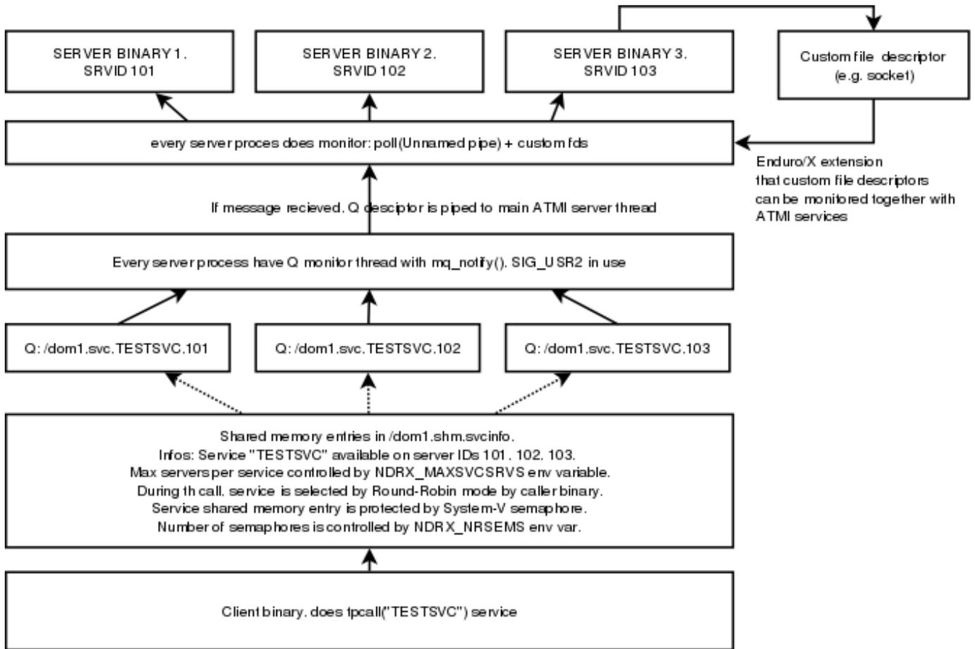
For other unix support, `mq_notify()` call for each open queue is installed, by employing `SIGUSR2`. Signal handling is done in separate thread. The main ATMI server thread is doing `poll()` in unnamed pipe. When event from `mq_` sub-system is received, it writes the queue descriptor id to unnamed pipe and that makes main thread to wake up for queue processing. The `poll()` for main thread supports Enduro/X extensions to add some other resource for polling (e.g. socket fd.)
