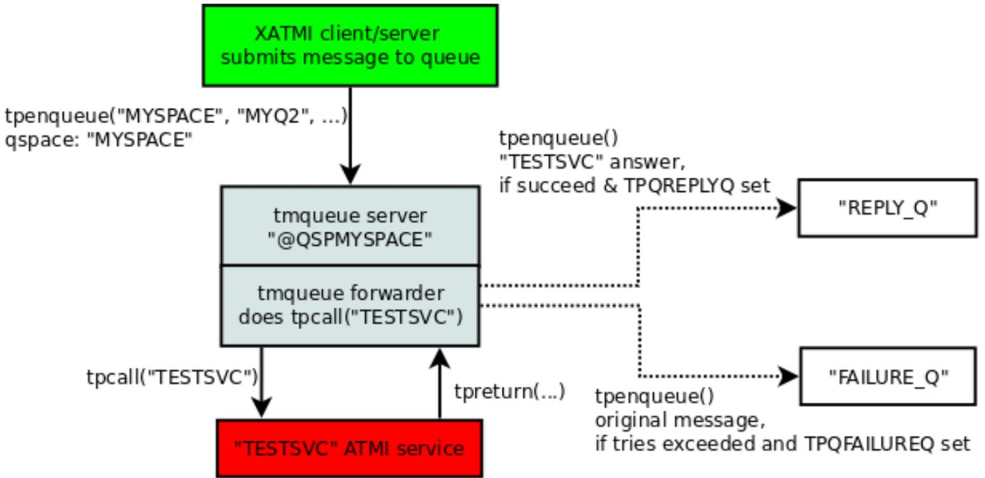
For `tpenqueue()` and `tpdequeue()` passed in buffers must be allocated with `tpalloc()`. For UBF, STRING and JSON buffers, the actual buffer length on enqueue doesn't matter, it is detected from data data inside. For array buffer, it does play a role. When doing `tpdequeue()`, the the buffer type might be changed, if message have a different data type.
