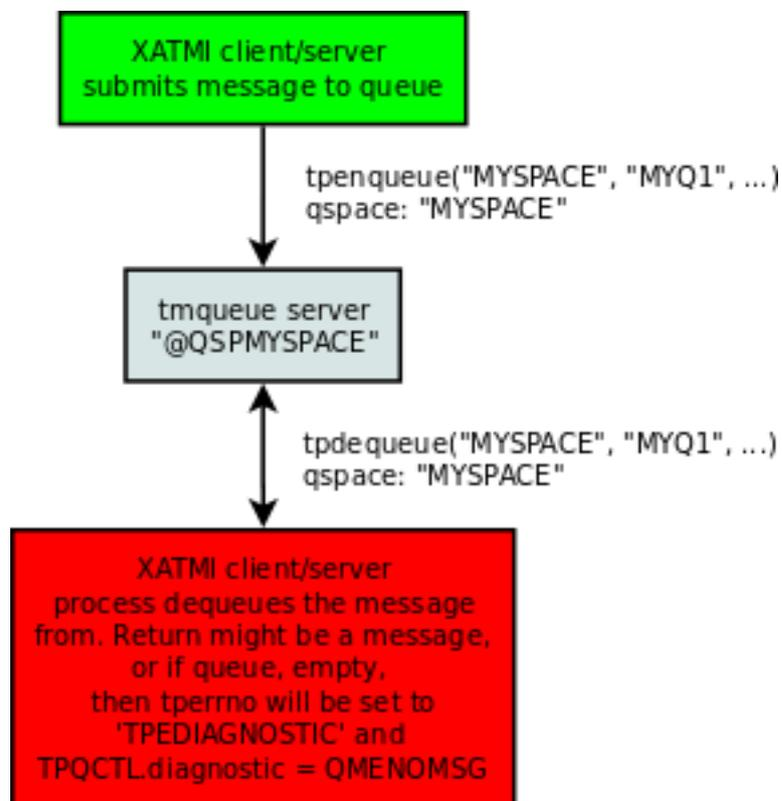
And another use is that process does `tpenqueue()` to automatic queue, and message is automatically forwarded to destination service. The schematics looks like this:
